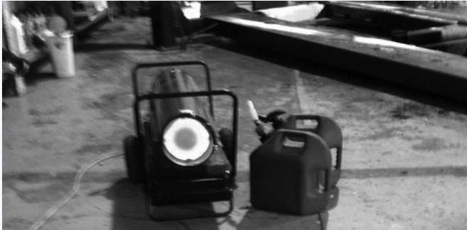
Even a blurry photo can't obscure the danger of placing a kerosene heater inches away from fuel containers. Hopefully, the containers are empty; but even if they are, they may emit flammable vapors that heat from the device could cause to ignite. The electrical cord stretching across the floor as a trip wire/additional source of ignition adds insult to injury.
